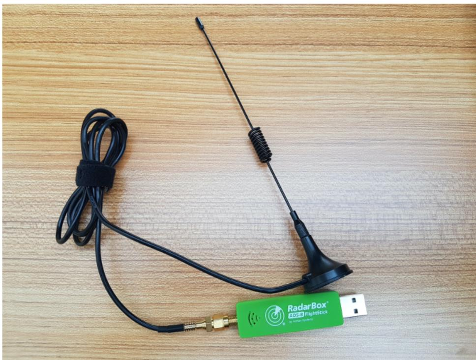
**Figure:** A USB-receiver which is capable of processing ADS-B (*Automatic Dependent Surveillance-Broadcast*) radio transmissions.
